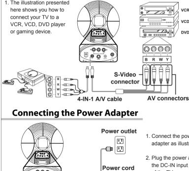
2. The cables are color-coded (black, red, white, and yellow). Connect each colorcoded cable to the appropriate connector on your
